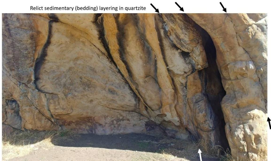
Figure 1: Evidence of steeply inclined bedding planes – this rock is a boulder, not in-situ bedrock. R. Cayley, GSV, June 2020
